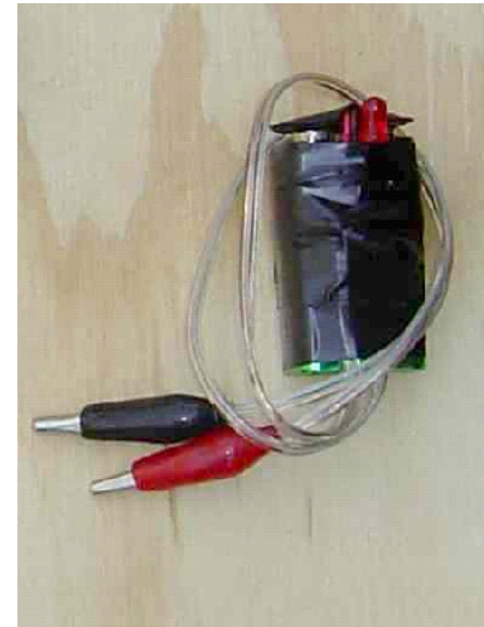
Electrical tape is used for final assembly
