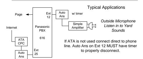
This design allows you to call in from the outside, either VOIP or POTS line and connect to your PBX. You can then dial numbers on your PBX, page or listen in to sounds in your yard. Ext 25 MUST be programmed NOT to allow access to outside lines. Auto Ans on Ext 12 must have a timer to properly disconnect. PBX does not provide a CPC pulse.
