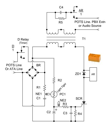
The neon lamp is to be glued to the photo cell. The back of the lamp (side not glued to the cell) is to be painted with white out, to reflect light to the cell. The "assembly" is covered in black electrical tape and made light tight. It will look ugly, but this is good. A double wrap of tape is best and very light tight.
