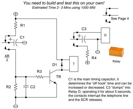
$R1, R4-47 \ Ohms-Limit \ charge \ current \ to \ capacitor \qquad R2-220K$   $R3-100K-Base \ Current \ limiter \qquad C1-Aprox \ 1000 \ Mfd \ 25 \ VDC$   $C2-0.1 \ Mfd \ 100 \ VDC-RF \ Filter \qquad C3-220 \ Mfd \ 25 \ VDC$   $T \ and \ D \ Relays-12 \ VDC \ Dip \ Package \ DPDT \ Aprox \ 700 \ Ohms$   $TR-2N4401 \qquad D1-1N4004$
