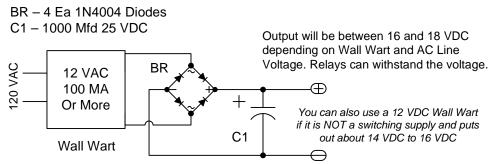
You can add an LED with a 1000 Ohm resistor across C1 if you want an indicator to show the power is on. The same can be wired on the second contact of Relay T to indicate Off Hook.
